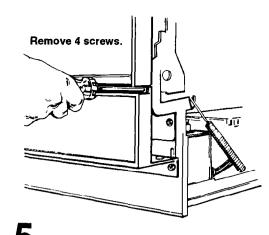
**O** Remove the 4 screws attaching access panel and toe panel to dishwasher using a 1/4" hex socket, nut driver or Phillips screwdriver. Remove access panel and toe panel.
